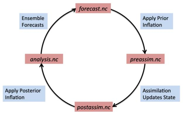
As shown here, an ensemble forecast is stored in forecast.nc, to which prior inflation can be applied and stored in preassim.nc. Once assimilation is applied, the output can be stored in postassim.nc, and finally if posterior inflation is applied, the final analysis can be written in analysis.nc. The model forecast will start from the analysis to advance the model in order to start the cycle over again.
