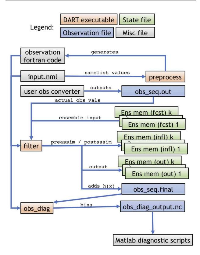
The single time-step workflow for an OSE experiment within a single step is slightly simpler than the OSSE equivalent as DART handles less of the process. Like the OSSE case, the namelist and preprocessed observation source files are input to all other DART programs. In the OSE case, however, the user must provide an **obs converter** that will output a obs\_seq.out file. There are many DART utilities to make this process easier, but for the OSE case
